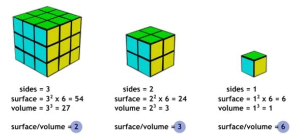
Figure 3: The relationship between particle size and surface area
