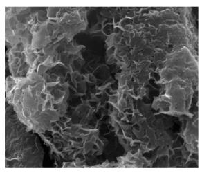
Figure 1: Porous nature of activated carbon.
