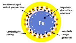
Figure 1. Schematic diagram of iron oxide-gold coreshell nanoparticle presenting electrostatic charges within each layer.
