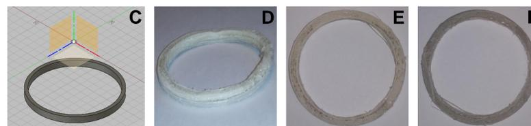
**Fig. 2.** Schematic showing the key components of a (A) hot melt extruder and a (B) 3D printer based on FDM technology; and the (C) computer aided design (CAD) for a vaginal ring (outer diameter 54 mm, inner diameter 50 mm, height 4 mm) which was used to 3D print (D) a combination ring with two discrete layers loaded with either (E) DPV 20% w/w or (F) LNG 20% w/w
