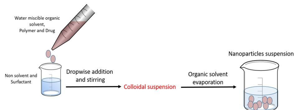
Figure 1: Nanoparticles manufacturing using nanoprecipitation method
